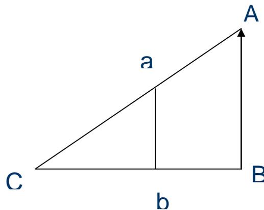
$$\begin{aligned} AB/ab &= BC/bc, \\ AB &= ab \times BC/bc \end{aligned}$$
