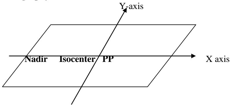
Fig 2: figure 2 showing the location of the PP, isocentre, and Nadir on a slightly tilted vertical APs
