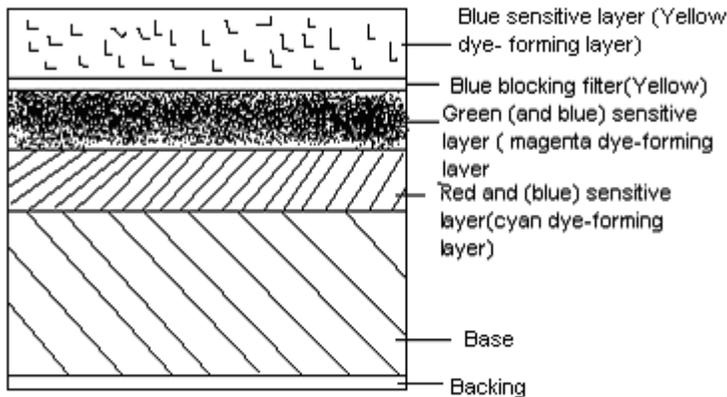
Fig: Generalised cross section of color film.
