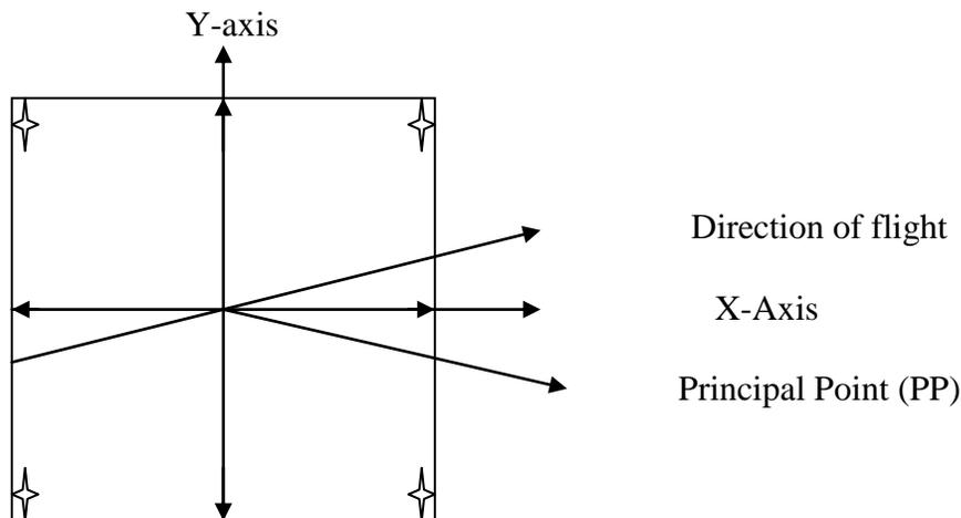
Fig: 2a Showing the fiducial marks, Principal points and co-ordinate axes of a single Aerial photo
