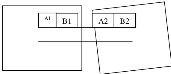
Fig: Parallax caused by improper orientation of the photos:
