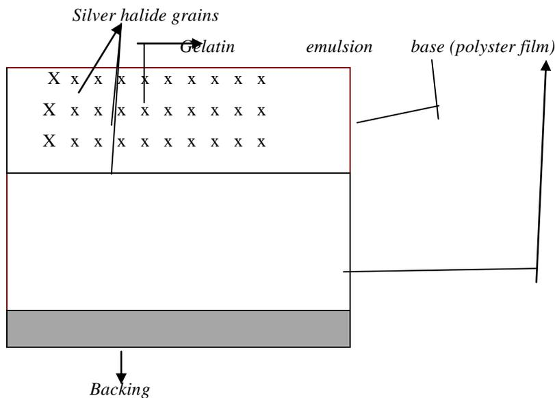
**Fig :( a) cross section of Panchromatic black and white film**
