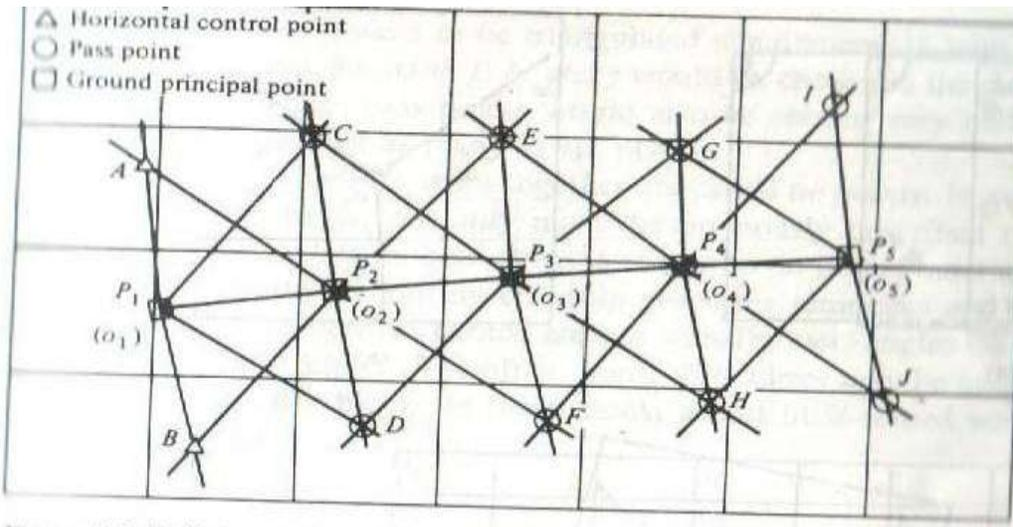
Fig 3: Radial-line triangulation assembly of five-photo strip
